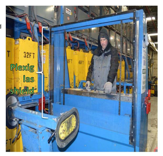
**After:** A large Plexiglas shield was installed on the battery changing machine between the operator and the batteries being changed, eliminating the hazard and the need for PPE.
