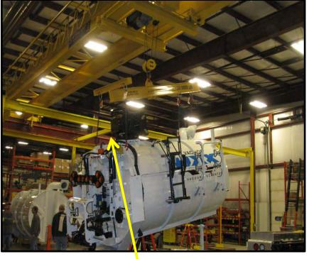
Designed a T-bar to lift the debris body. Lift chains no longer come in contact with turret or debris body
