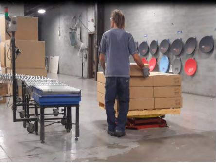
Material Handlers palletized 10-pack boxes of satellite dishes manually. This required frequent lifting of 45 lb. boxes above shoulder height and carrying of the boxes around the pallet to stack on the far corners of the pallet. Installation of the PalletPal eliminated the walking and carrying due to the rotating turntable, and reduced above-the-shoulder lifting due to the spring-adjusted height of the platform.
