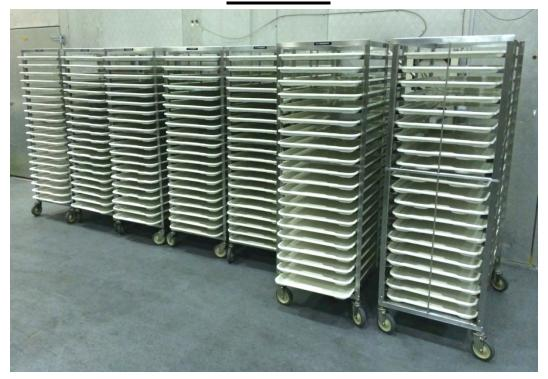
Various replacement options were researched and a suitable food grade smooth edge fiberglass tray was found. 600 New trays and 27 custom stainless steel carts were procured to completely replace/retire unsafe equipment. Total cost Approx. \$100,000.
