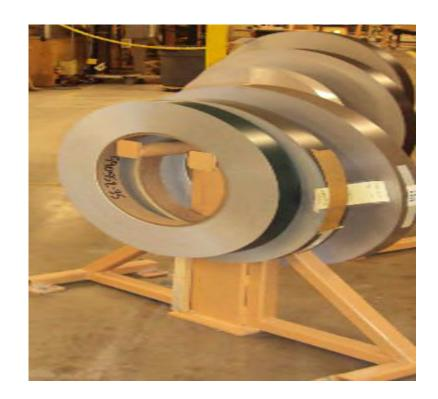
Stands were built to keep the coil off the floor.
