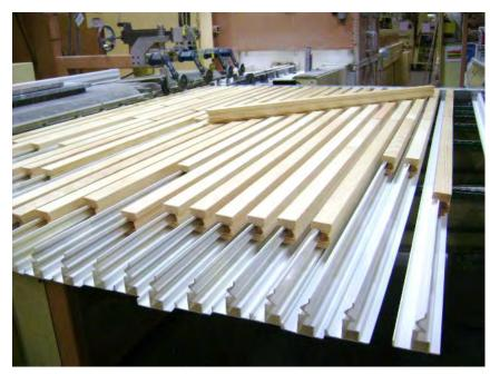
Trays were developed for the parts to be pulled directly from the kitting carts onto the infeed of the Paintline. Ergonomically friendly to use, by snapping the part on and off the tray with a simple pinch and twist of the wrist.
