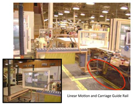
Roller system was built on so that the units can now be loaded onto the skid after passing down the moveable roller system. This is realigned for each unit onto the skid making minimal effort needed from the Team Member.
