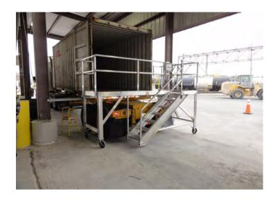
After – Had contractor fabricate large aluminum platform with stairs.
