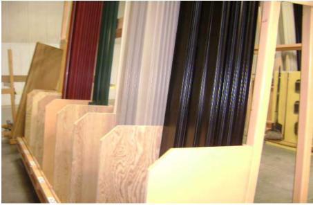
Vertical racking was installed in the area, we staged our lower volume color offerings staged in it. This helped us eliminate the reaching for our Team Members.
