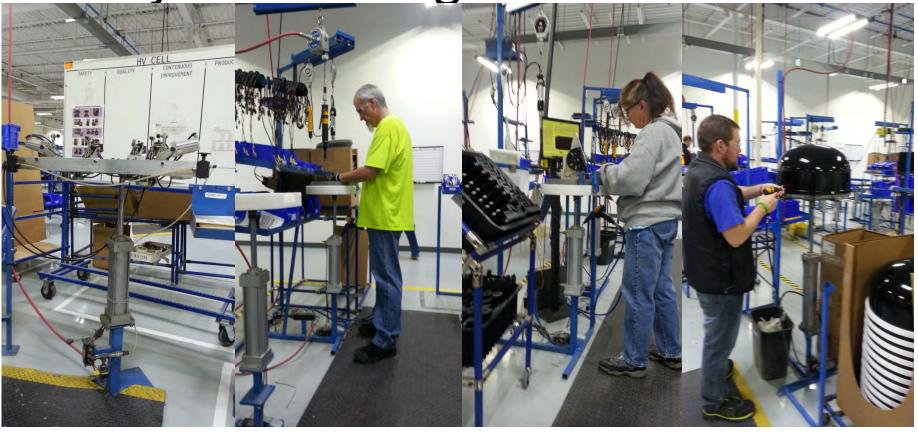
Adjustable height work stations are made by placing a pneumatic cylinder in line between the base and assembly fixture of the work station. Adjustable height allows employees of different heights to work with their backs and upper extremities in neutral postures during assembly operations. The height of the work station is easily altered with an actuating lever so that the height of the work station can be changed to optimize posture for each step of the assembly operation.
