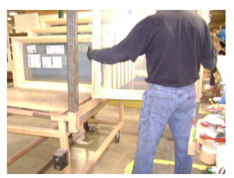
Team Member needed to lift units off the assembly table, carry a short distance and place onto shipping skid. Ergonomic Concerns included lifting, twisting and frequent size change. After
