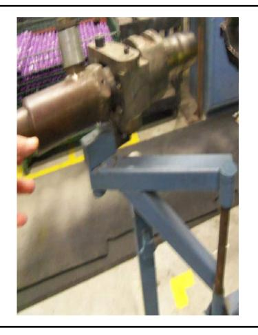
When loading a reel the associate had to make sure the reel flange notches were lined up with the drive arm which rotated during operation and could catch an associate. A flange was added to secure the reel in place and the drive arm was removed eliminating the hazard of rotating parts. This change improved the process while making it safer.
