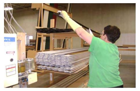
As our product offering continue to grow, so did the height of our lineal extrusion carts. Team Members were consistently reaching above their heads through out the shift to pull down the extrusion and stage on the saw.
