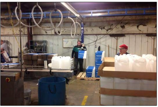
During this offseason Tim Klaver, our Specialty Production Manager installed a vacuum lifting system to eliminate the repeated exposure to back injuries from manually lifting the boxes and stacking the heavy boxes on a pallet.
