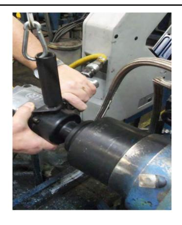
Associates had to manually remove a the pin holder and move it to a table near them. The pin holder weighs approximately 70 pounds. A pin holder swing arm was installed that attached to the pin holder eliminating the need for manual lifting. The swing arm allows the associate to shift the pin holder out of the work area to complete their task and swing it back into place when job is completed.
