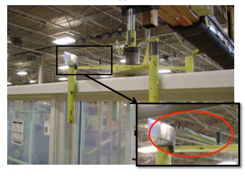
Process required Team Member to hold edge board in place causing a potential pinch point. Or the other option was to have another Team Member in the area to help Secure the packaging at the start of the wrapping process.
