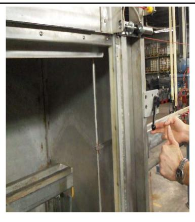
Associates had to manually remove a die nut to change a die. Back strains were reported due to the weight of the wrench and the force required to remove the die nut. An impact wrench was added with the use of a counter balance so associates wouldn't have to lift the weight of the impact wrench. Back strains were eliminated after implementation.
